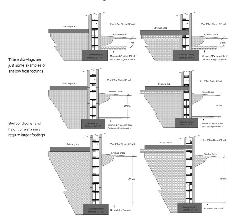
Contractors must check and follow local codes when using shallow frost footings.
